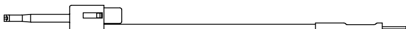
PICO-HOOK, LEAD WIRE DESCRIPTIONS AND COLOR CHOICES: See Basic PICO HOOK. .025" (.635mm) SQUARE PIN PLUG: Gold-Plated Brass Body. Heat Shrink Insulator. Crimp Assembly. See P/N 9265-HS.
